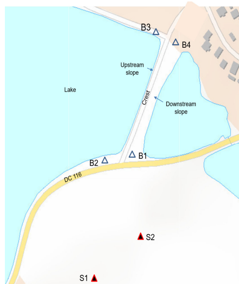
Figure 7 - Geodetic monitoring network designed for the Podisu dam
