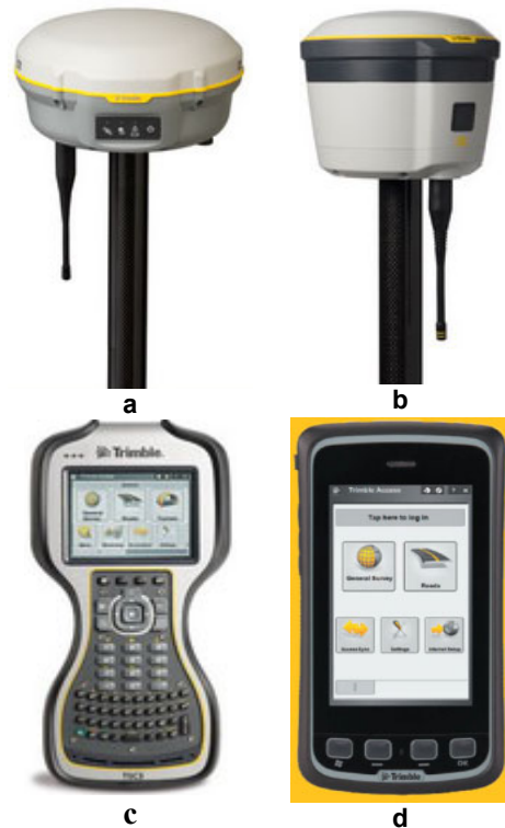
Figure 5 - GNSS equipment used for measurements: a - Trimble R8S receiver; b - Trimble R2 receiver; c - Trimble TSC3 control unit; d - Trimble Slate control unit
