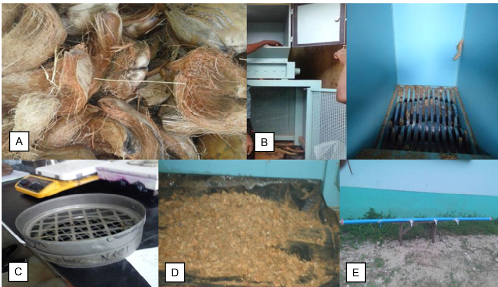
A = Dried coconut husks; B = shredder; C = sieve; D = sieved coconut husks; E = purification column
