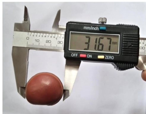
Figure 1 - (a) Representation of the three perpendicular dimensions of Dioclea reflexa seed. (b) Dimensional seed measurement with Vernier caliper
