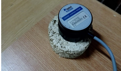
Figure 7 – Measuring the heat transfer coefficient
