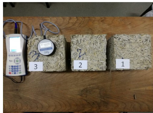
Figure 5 - Measurements of the heat transfer coefficient
